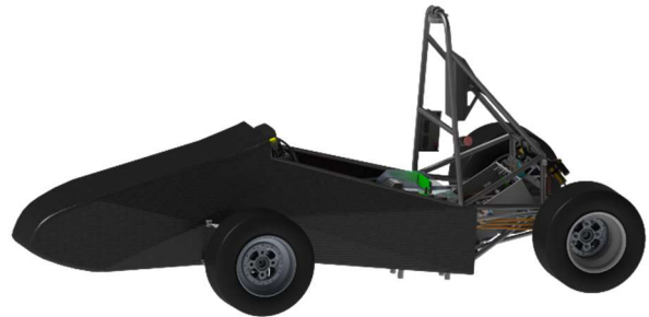
Figure 7: Reduced aerodynamic design to body panel (deadline pressure)
